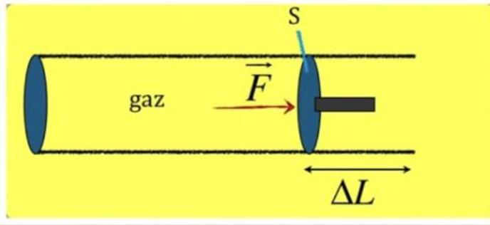
$$W = \vec{F} \cdot \vec{l} = F \times \Delta L = P \times S \times \Delta L = P \times \Delta V$$
